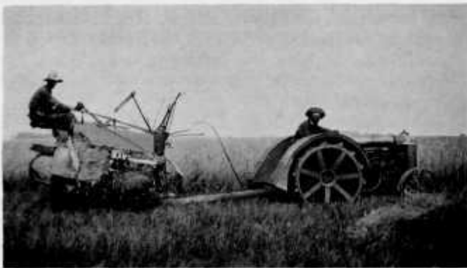
Cutting wheat in Norway Township about 1932. Henry Nysveen on a 1927 Fordson Tractor pulling a Minnesota eight foot binder with Ottar Sliper at the controls.
